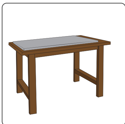
Stable Work Table With Sacrificial Board/Fiber Cement
