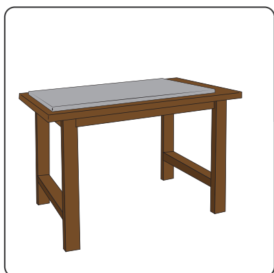
Stable Work Table With Sacrificial Board blade
